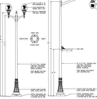
16.5' Pole with double Acorn fixture for use along Main Street, 100' o.c. typ.
