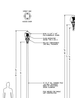
14' Pole with Acorn Fixture, similar to existing luminaires, for use along Main Street, 50'
