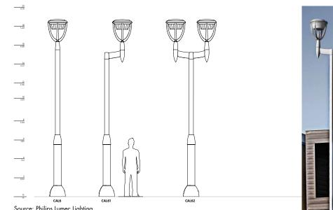
Lighting Alternative: Philips Lumec Callisto lantern series. Pole height can be specified between 8-18 feet tall, at 6" increments.
