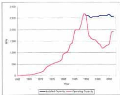
Figure 1 California Installed and Operating Geothermal Capacity 4 (1960-2003)
