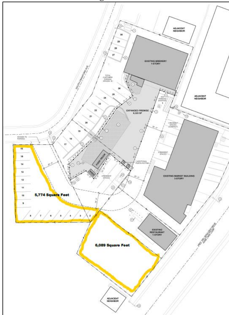
FIGURE 5. Snow storage areas
