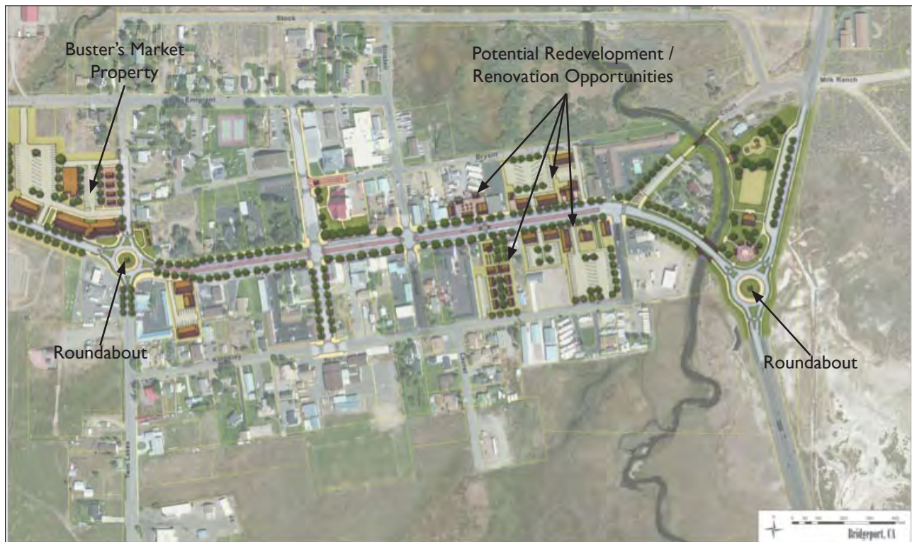
Figure 3. This is an idealized overview of a possible long-term design for Bridgeport. Note that it includes redevelopment of the Buster's Market area, roundabout gateways, reuse of underutilized properties along Main Street, and an increase in facilities at the ice pond site. These enhancements all need further discussion, engineering, and evaluation before they can be realized.
