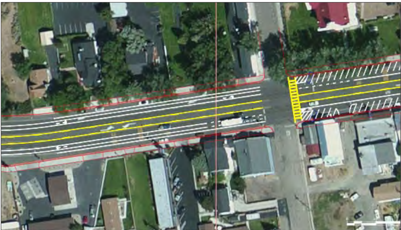
Figure 13. Parallel parking will remain in place west of School Street, but reverse angled parking will be striped east of that intersection.
