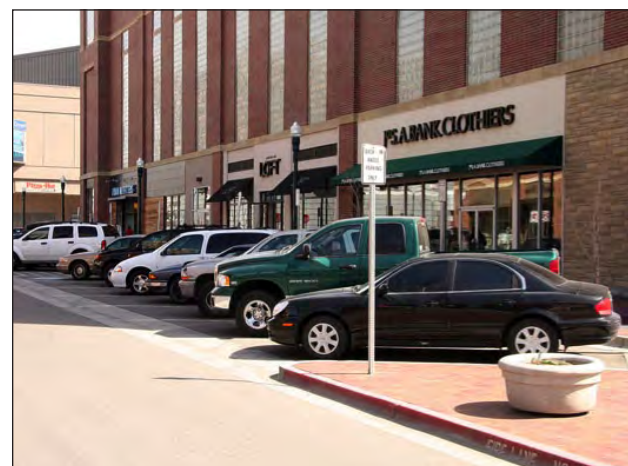
Reverse angle parking gives drivers a better view, and allows cargo loading from the sidewalk.
