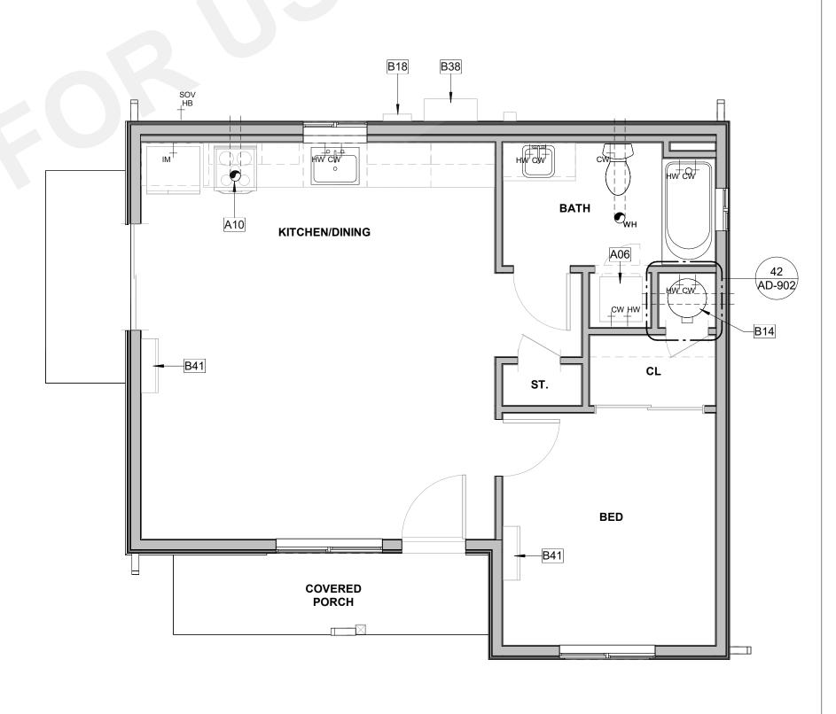
2 GROUND FLOOR PLAN - MECHANICAL A1-201 A2-111 SCALE: 1/4" = 1'-0"
