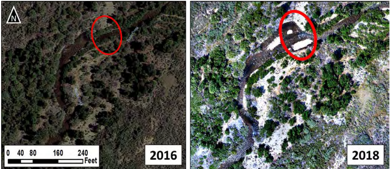
Figure 16. Aerial imagery of the same stream section in Rush Creek showing change in channel morphology from 2016 (Google Maps, 2019) to 2018 (Adair, 2018). The red circle marks the location of a measured active channel width at a riffle crest, showing how the channel widened into the left bank following the RY2017 flood hydrograph.
