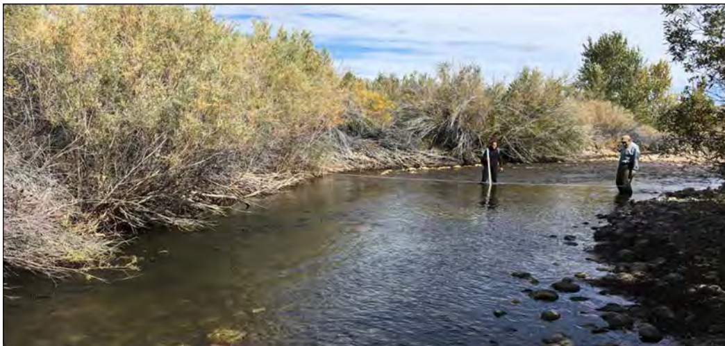
Figure 8. Emily Cooper (left) measured the riffle crest thalweg depth to the water's surface along a surveyor tape stretched out the length of the active channel width in Rush Creek. Bill Trush (right) recorded these measurements (Photo: 1 Oct., 2019, 11:24 AM).
