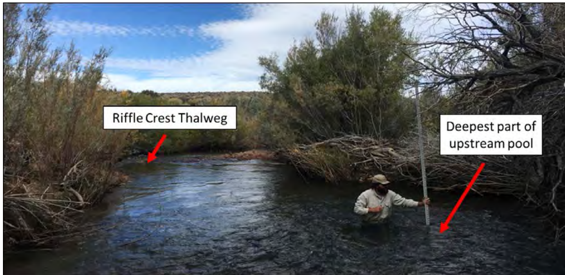
Figure 18. Mason London measuring the deepest location in a pool upstream of an already measured riffle crest thalweg in the lower mainstem reach of Rush Creek. (Photo taken 29 Sept, 2018, 10:46 am).
