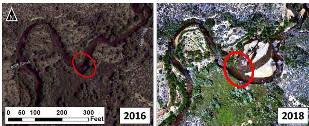
Figure 17. Aerial imagery of the same reach in Rush Creek showing change in channel morphology from 2016 (Google Maps, 2019) to 2018 (Adair, 2018). The red circle marks the location of a measured active channel width at a riffle crest, showing how the channel widened after 2017 peak flows. Note that the riffle crest in 2018 (with an active channel width at its location of 63.3 ft.) was newly formed and therefore there was not a corresponding measurement recorded in 2016. This channel bend is located in the lower portion of the lower mainstem reach within Riparian 2.
