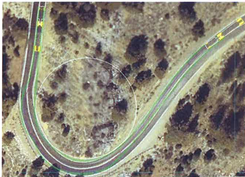
MNO 108 – Example of Truck Off-Tracking at PM 7.0
