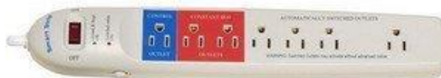
Figure 5.5: Sample Smart Power Strip – Blue Outlet Is “Master”, White Outlets Are Controlled, Red Outlets Are “Always On”
